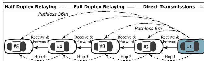
Figure 1. Overview of our five-vehicle platoon model. The figure illustrates the three considered communication scenarios of Half Duplex Relaying (HDR), Full Duplex Relaying (FDR), and Direct Transmission (DT), for beaconing in platooning.
