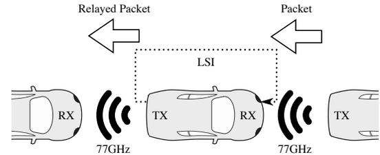
Figure 1. FDR in a platoon: The first vehicle transmits a packet via RADCOM. The signal is amplified by the intermediate vehicle and transmitted from its back. Due to reflections, part of the signal can be received by the intermediate vehicle during relaying, inducing LSI.
