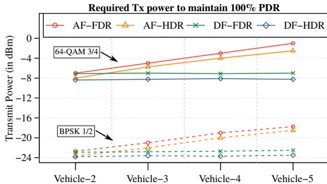
Figure 4. Required transmit power from the leading vehicle for the considered AF and DF relaying schemes, to maintain a 100% PDR using a 77 GHz mmWave link, operating in both HD and FD mode. For visual clarity, the plot only shows the data for the lowest and highest MCS at each relaying vehicle.
