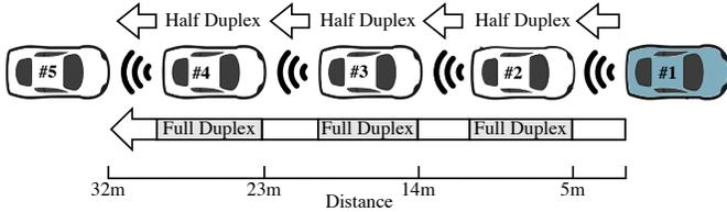
Figure 2. The simulation scenario: A platoon of five vehicles that uses either HDR or FDR. Arrows indicate transmissions. With HDR relaying four individual transmissions are needed, while FDR relaying only requires one. The scale at the bottom indicates vehicle distances from the leading vehicle.
