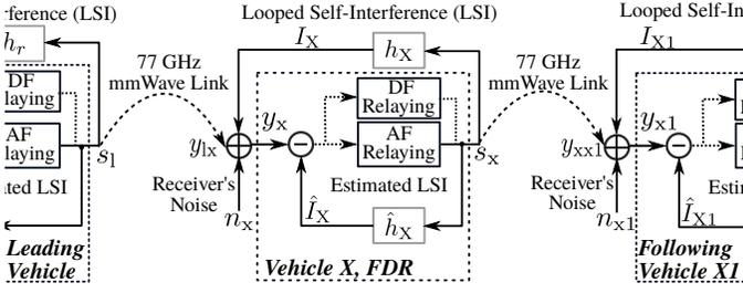
Figure 3. Block diagram for modeling the LSI in vehicle platoons. The model here shows three vehicles, i.e., leading vehicle, vehicle X, and following vehicle X1, in a multi-hop FD relaying network. Each relaying vehicle is capable of performing both AF and DF relaying schemes.
