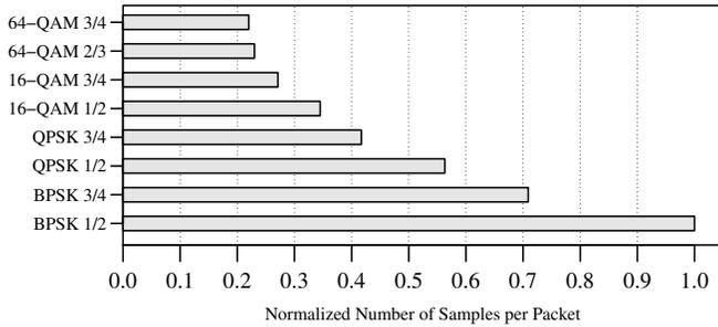
Figure 6. Normalized packet length for sending the same payload with different modulation and coding schemes.
