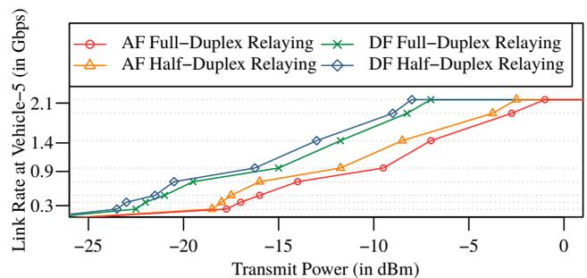
Figure 5. Achievable bit rates at the last vehicle (Vehicle-5) for 77 GHz mmWave link with 800 MHz bandwidth, in the considered Half Duplex Relaying (HDR), Full-Duplex Relaying (FDR) scenarios of vehicular platoon.
