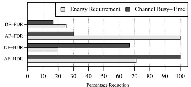
Figure 8. Reduction in the energy requirements and the channel busy-time in each employed relaying scheme under both FDR and HDR modes.
