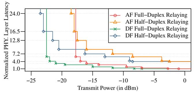
Figure 7. Normalized physical layer latency at the last vehicle (Vehicle-5) for 77 GHz mmWave link with 800 MHz bandwidth in the considered platooning scenario.
