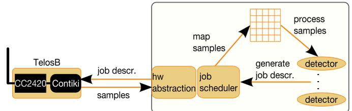
Figure 1. Interferer detection architecture
