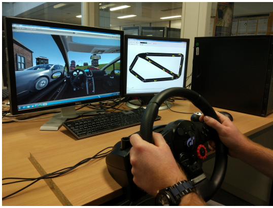
Figure 2. Overview of the demo setup. The driver is controlling the ego vehicle with the steering wheel. The left monitor shows his first person view from within the vehicle, the right monitor displays the VANET simulation.
