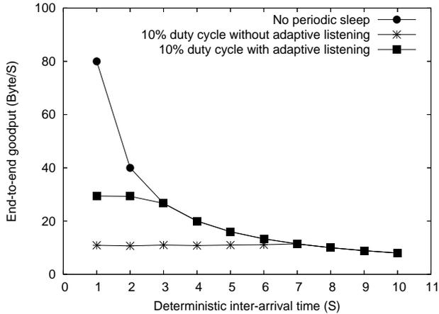
**Figure 6: Mean end-to-end goodput under CBR traffic source**
