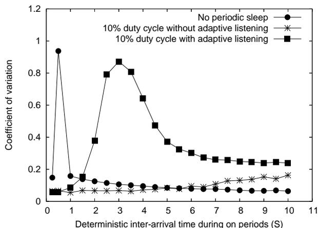
**Figure 9:** Coefficient of variation for end-to-end delays under the combination of CBR and On/Off traffic sources
