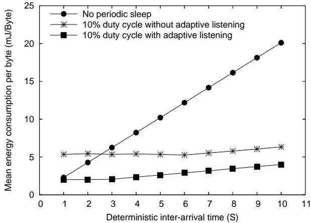
Figure 4: Mean energy consumption per payload byte under CBR traffic source
