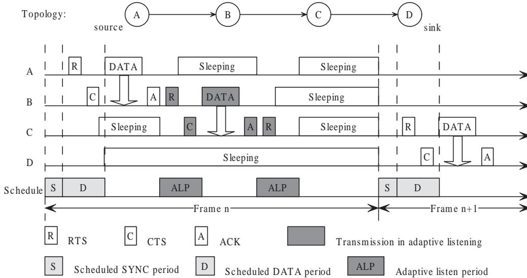
Figure 2: Transmitting a data packet through a three-hop network with adaptive listening
