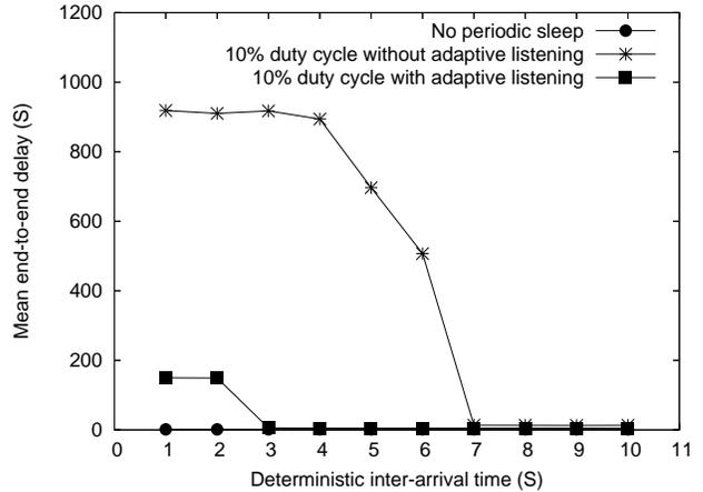
Figure 5: Mean end-to-end delay under CBR traffic source
