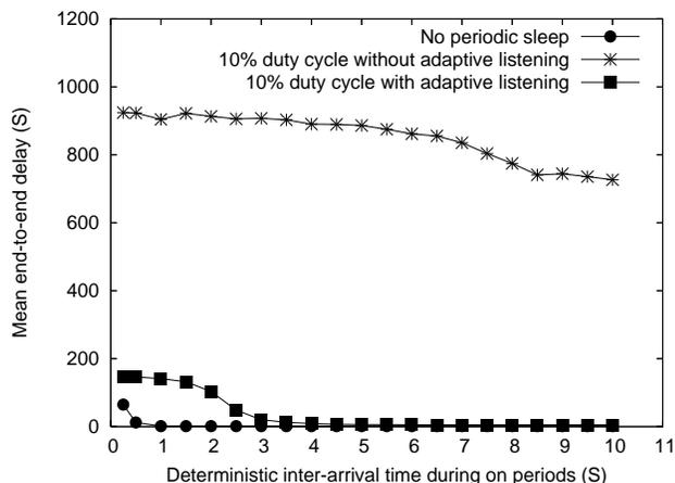
**Figure 8:** Mean end-to-end delay under the combination of CBR and On/Off traffic sources
