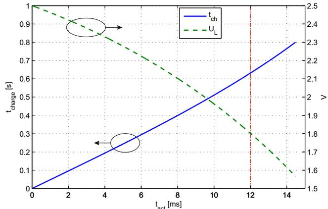
Figure 4. Dependency of the active period and the recharging time.
