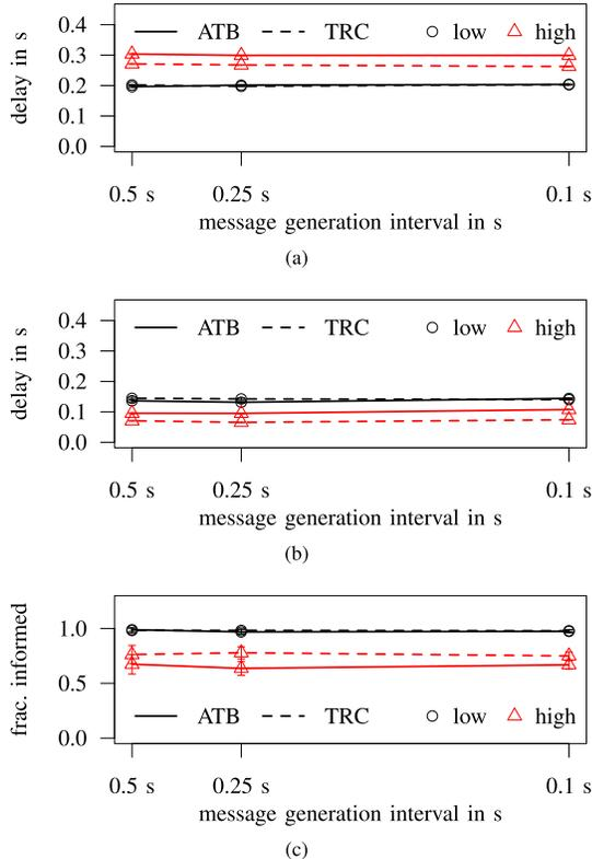
Fig. 8. Class C protocol performance for low and high density scenarios and different message generation intervals. Plotted are the results using the ATB and TRC Class A protocols; the results are comparable to 1 Hz beaconing. (a) Delay for Manhattan scenarios. (b) Delay for freeway scenarios. (c) Fraction of successfully informed nodes for Manhattan scenarios.
