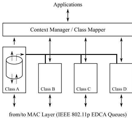
Fig. 2. System design overview. A context-aware class mapper coordinates data exchange of applications with four distinct protocols, each connected to the MAC layer using different priorities and each fulfilling a specific role.
