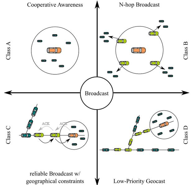
Fig. 1. Our vision of VANET broadcast classes: Class A for medium priority CAMs; Class B for forward highest priority events within  $N$  hops; Class C for high priority reliable broadcasting with geographical constraints; and Class D for low priority geocasting.
