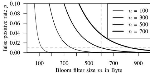
Fig. 3. False positive rate  $p$  of a Bloom filter as a function of its length  $m$  and the inserted element count  $n$ .
