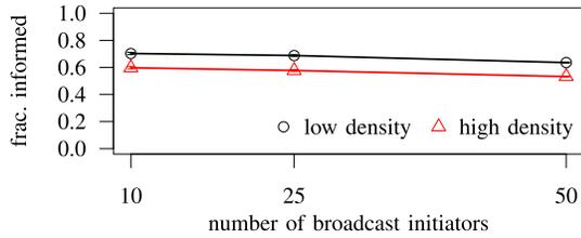
Fig. 7. Fraction of successfully informed nodes for low and high density Manhattan scenarios using a greedy approach for message dissemination. Plotted are the results using TRC as the Class A protocol and the Manhattan scenario.
