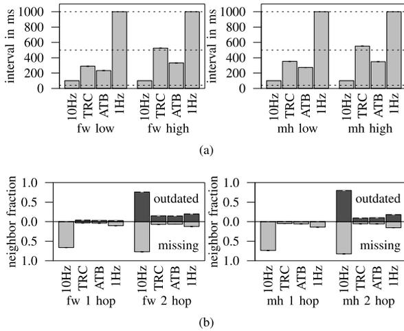
Fig. 5. Class A protocol performance for the freeway and Manhattan scenario and different vehicle densities. (a) Resulting beacon interval indicating the latency performance. (b) Neighbor ratio for 1-hop and 2-hop neighbors (high density scenarios).
