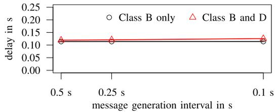
Fig. 11. Integrated Class A, B, and D performance (delay of Class B messages) for different message generation intervals; results plotted for using TRC as a Class A protocol and a high density Manhattan scenario; results for ATB and 1 Hz are comparable to TRC; results are similar for the freeway scenario.
