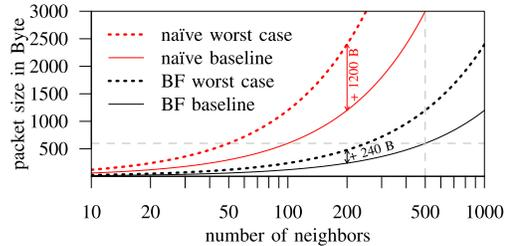
Fig. 4. Packet size for neighbor information as a function of the number of neighbors; for the Bloom filter (BF) approach we assume  $p = 0.01$ , and for the naïve approach we use 6 Byte per neighbor entry.
