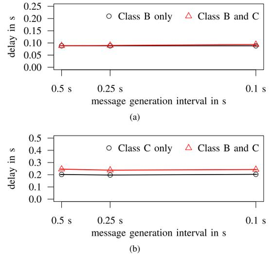
Fig. 10. Integrated Class A, B, and C performance for different message generation intervals; results plotted for using TRC as Class A protocol and a low density Manhattan scenario; results for ATB and 1 Hz are similar to TRC; results are similar for the freeway scenario. (a) Delay of Class B messages. (b) Delay of Class C messages.
