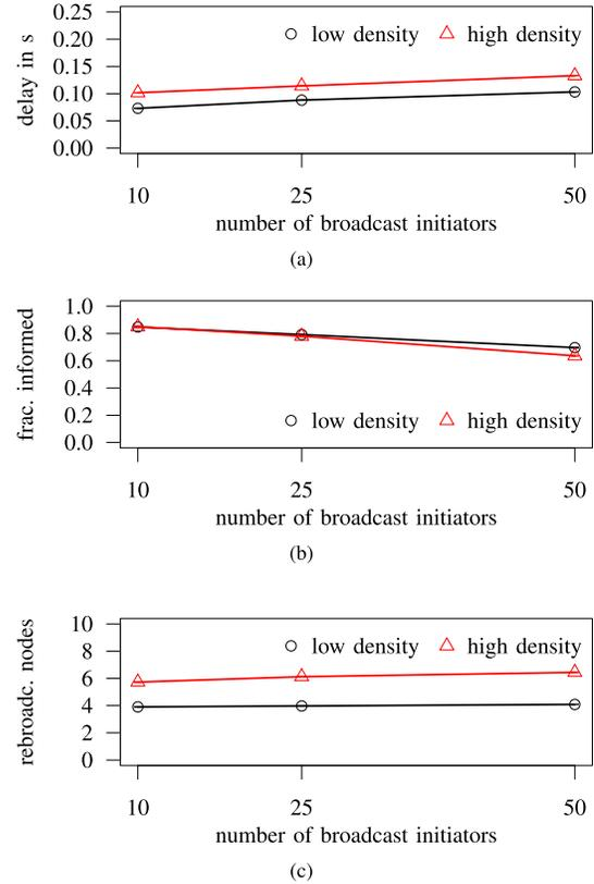
Fig. 6. Class B protocol performance for different numbers of broadcast initiators. Plotted are the results using TRC as the Class A protocol and the Manhattan scenario; results are similar for the freeway scenario. (a) Delay for low and high density Manhattan scenarios. (b) Fraction of successfully informed nodes for low and high density Manhattan scenarios. (c) Selected rebroadcast nodes for low and high density Manhattan scenarios.
