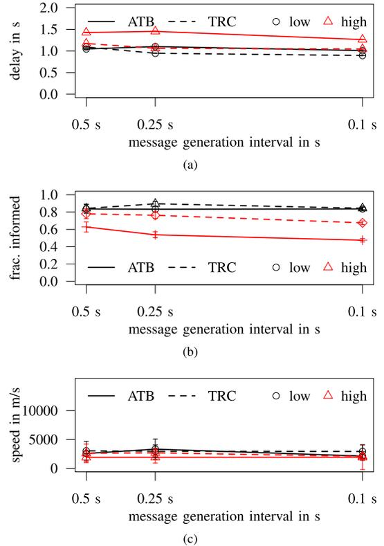
Fig. 9. Class D Performance for different message generation intervals in low and high density scenarios. Plotted are the results using the ATB and TRC Class A protocols; results for 1 Hz are comparable to TRC; results are similar for the freeway scenario. (a) Delay for Manhattan scenarios. (b) Fraction of successfully informed nodes for Manhattan scenarios. (c) Dissemination speed of new messages for Manhattan scenarios.
