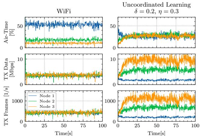
Fig. 5. Air-time allocation, individual throughput and packet rate in case of heterogeneous traffic, i.e., all nodes use the same packet size of 1500 B, but different data rates  $M_i \in \{6.5, 26, 65\}$  Mbps.
