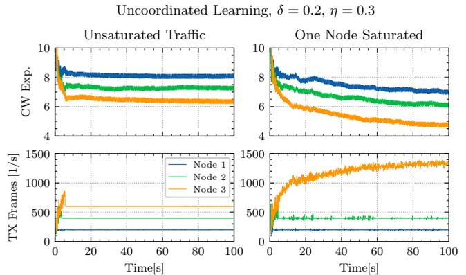
Fig. 8. Individual contention window and packet rate in unsaturated scenario (left) with offered load of  $r_i \in \{200, 400, 600\}$  pkts/s and with one node saturated (right), i.e.,  $r_i \in \{200, 400, 2000\}$  pkts/s.
