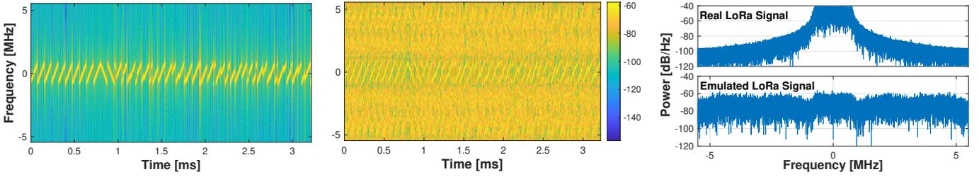
Fig. 8: Spectrogram of real (left) and emulated (middle) LoRa frames as well as their spectrum profiles (right).
