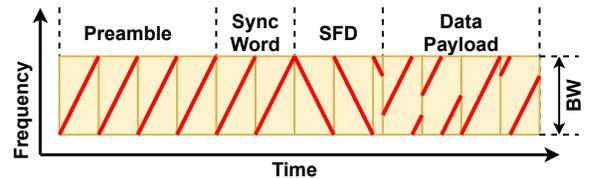
Fig. 4: Structure of LoRa Frame.
