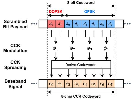
Fig. 3: 802.11b CCK scheme for data rate of 11 Mbit/s.
