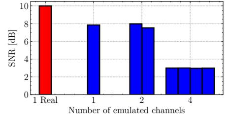
Fig. 11: SNR of multiple LoRa channels emulated in a single WiFi frame.
