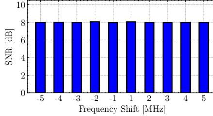
Fig. 10: SNR of an emulated LoRa signal shifted within the BW of a WiFi frame.
