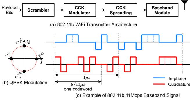
Fig. 2: 802.11b WiFi transmitter architecture (a), QPSK constellation diagram (b), and example CCK baseband signal (c).
