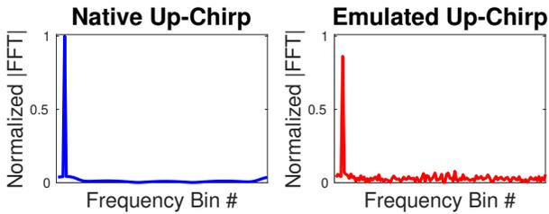
Fig. 7: Demodulation of real and emulated LoRa up-chirp.
