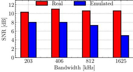
Fig. 9: Comparison of SNR of real and emulated LoRa signals.
