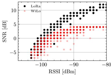
Fig. 12: Comparison of RSSI and SNR of real and emulated LoRa signals in an over-the-air experiment ( $SF = 6$ ).
