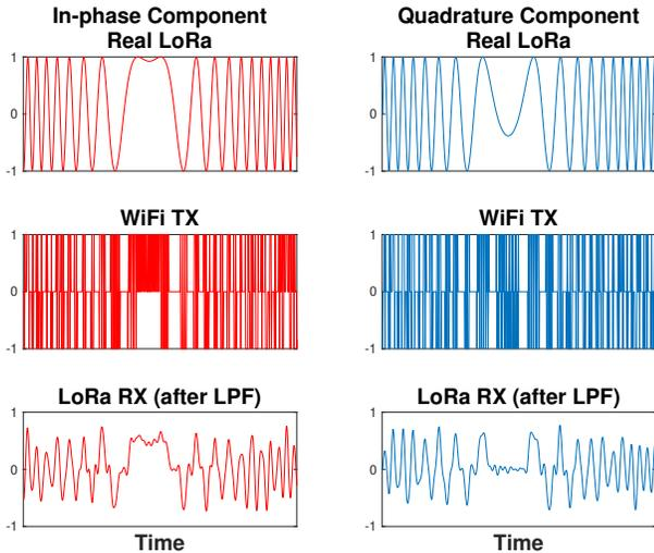
Fig. 6: Emulation overview: real LoRa up-chirp, WiFi waveform and signal received by LoRa device (after LPF).
