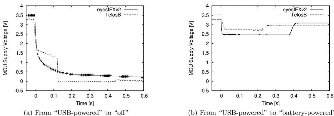
Figure 3.3: Time response of the sensor node MCU supply voltage after the respective USB hub has received a port power-control command from the testbed
