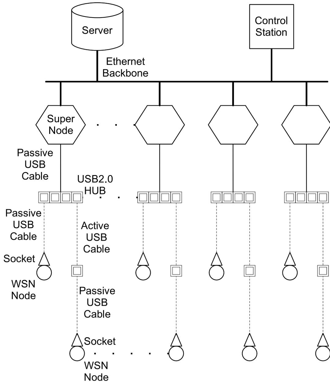
Figure 3.1: Hardware architecture of the TWIST testbed
