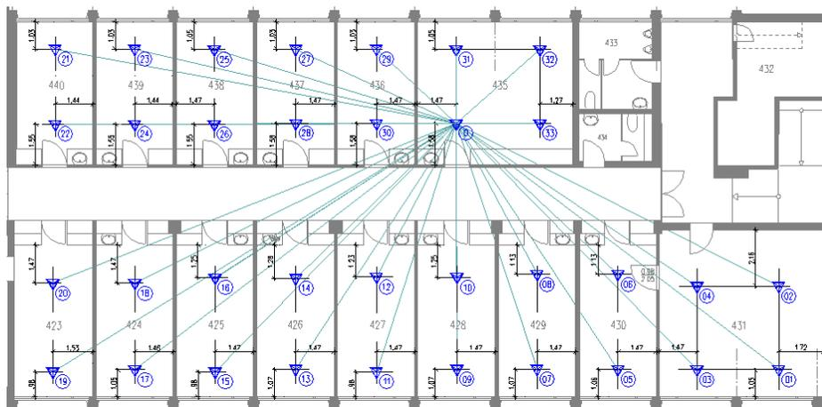
Figure 4.1: Node placement on the 4th floor
