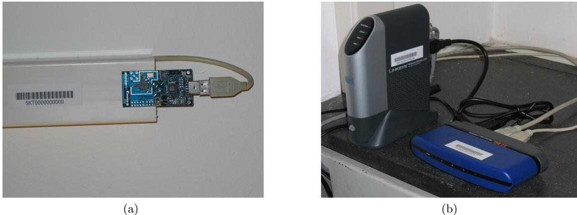
Figure 3.2: (a) Telos mote in a testbed socket; (b) Super node and USB-hub arrangement
