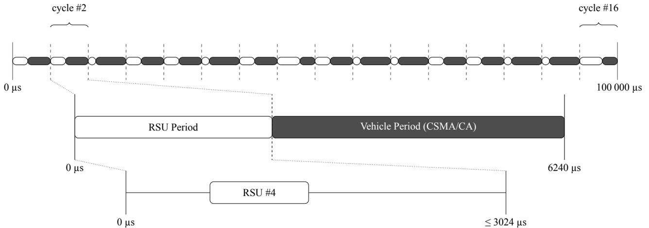
Figure 2. The 100ms control cycle for transmission control which is split into 16 smaller cycles. Those cycles are again divided into two parts by the TDMA scheme. Within those parts a second channel access coordination among nodes of the same type is done.
