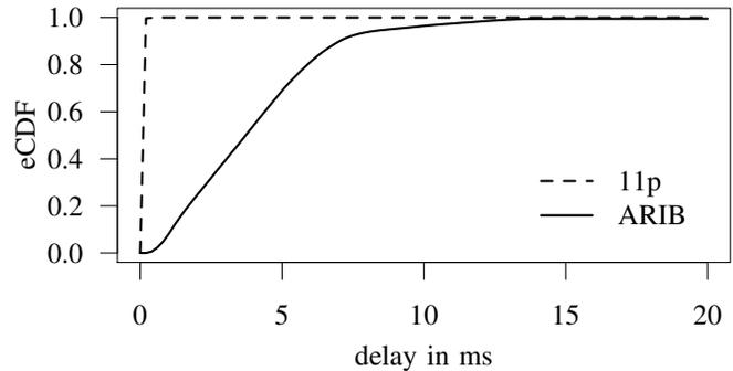
Figure 12. The delay of ARIB T109 in comparison to IEEE 802.11p.
