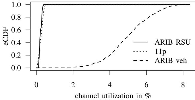
Figure 9. The MAC utilization of ARIB T109 in comparison to IEEE 802.11p.
