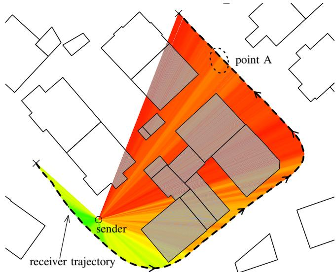
Figure 4. A map around Andreasstraße in Paderborn where we conducted our measurements: The colored lines show the signal strength for 868 MHz along the receiver trajectory. At *point A* a small LOS corridor leads to an increased signal strength.
