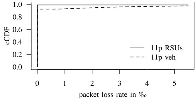
Figure 11. The packet loss rate of frames sent by RSUs and vehicles in IEEE 802.11p.
