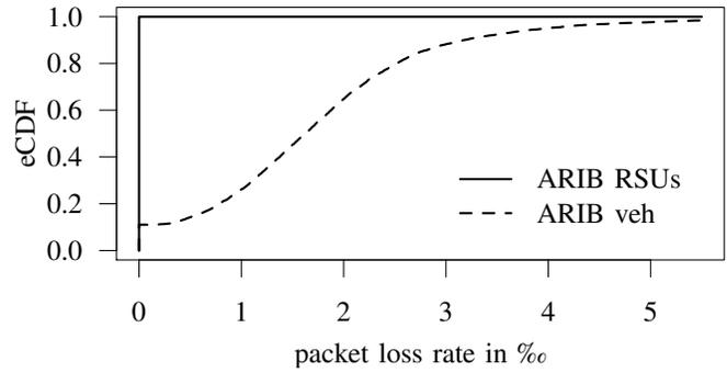
Figure 10. The packet loss rate of frames sent by RSUs and vehicles in ARIB T109.
