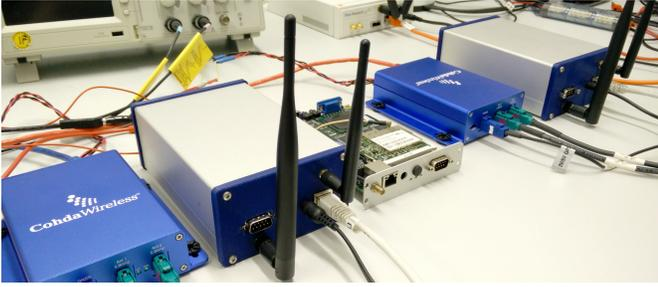
Figure 1. Devices used in the experiments: embedded systems running Linux 3.9, outfitted with a UNEX DCMA-86P2 miniPCI card using the ath5k driver, and Cohda Wireless MK5.
