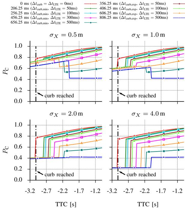
Fig. 4.  $P_C$  over time for different position inaccuracies ( $\sigma_x$ ) and different delays, starting at -3.2s before the collision.
