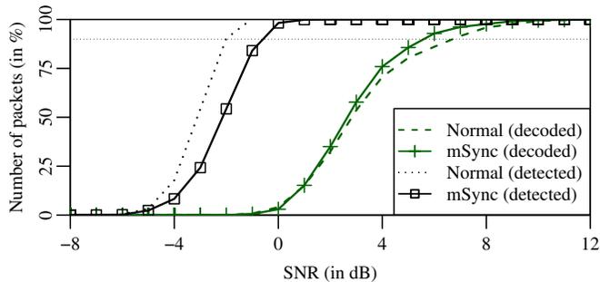
Figure 2. Packets detected vs. correctly decoded over an AWGN channel.
