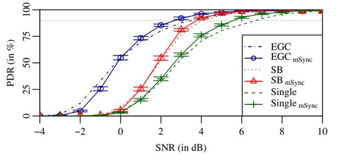
Figure 3. Simulated performance of mSync and normal approach with diversity combining over an AWGN channel.
