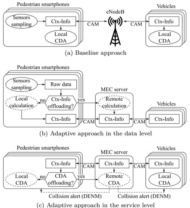
Figure 2: MEC-based Collision Detection.
