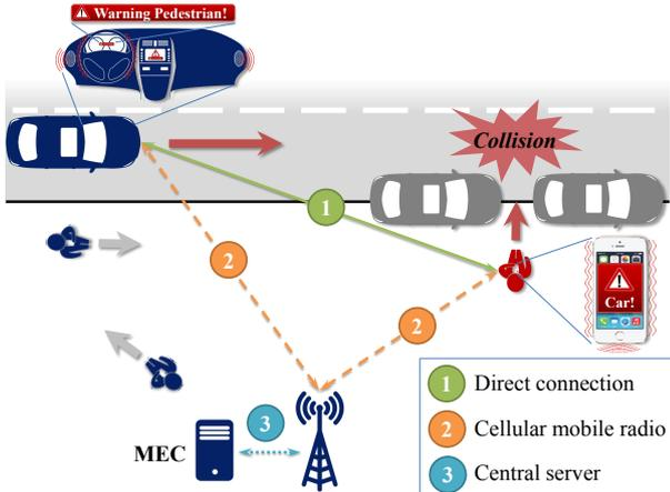
Figure 1: General concept of a VRU safety system.
