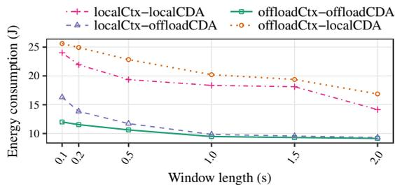
Figure 6: Energy consumption vs. operation schemes ( $f = 50$  Hz).
