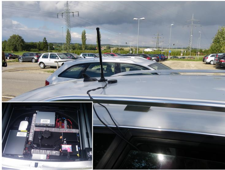
**Figure 3.12** – Position of the shark fin antenna assembly, omnidirectional antenna, and GPS receiver used for signal attenuation measurements; inset: installation of the DENSO WSU 802.11p radio in the trunk.
