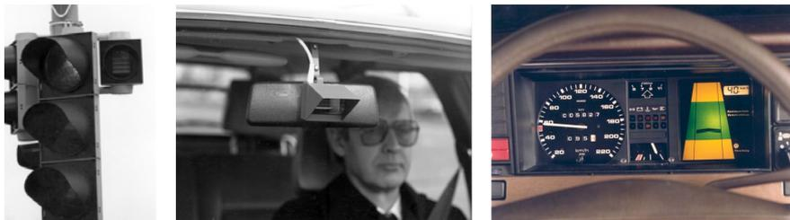
(a) infrared sender at a traffic light (b) infrared receiver mounted on rear-view mirror of an equipped vehicle (c) traffic light phases and speed recommendation shown in the vehicle
