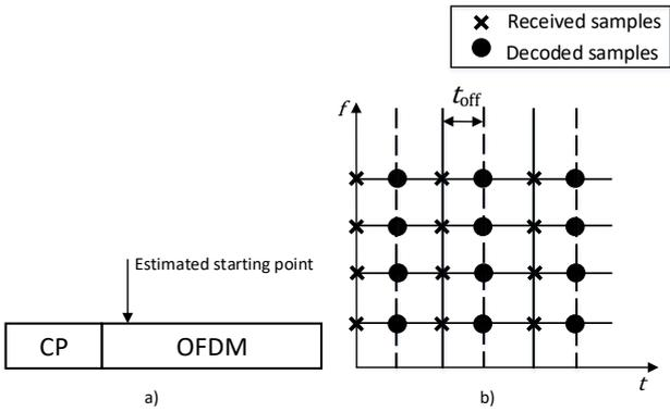
Fig. 1: Example of symbol timing offset effect. a) Received OFDM symbol. b) Effect on the time-frequency domain.
