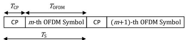
Fig. 4: Estructure of transmitted OFDM symbols.
