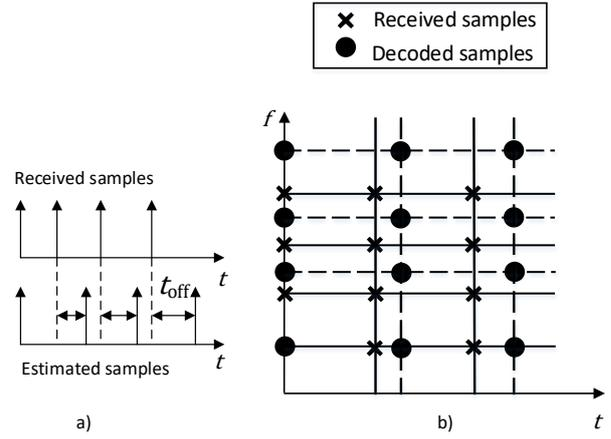
Fig. 3: Example of clock frequency offset effect. a) Time representation of sampling clock frequency offset. b) Effect on the time-frequency domain.
