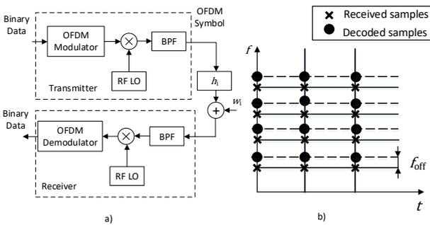
Fig. 2: Example of carrier frequency offset effect. a) Transmitter and receiver schemes. b) Effect on the time-frequency domain.
