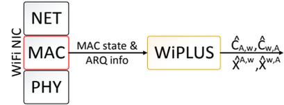
Fig. 4: WiPLUS is based on MAC layer monitoring.
