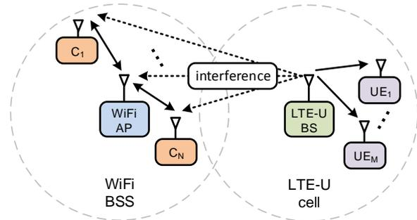
Fig. 3: System model — WiFi BSS co-located with LTE-U cell. The LTE-U DL traffic creates interference on WiFi BSS DL and uplink (UL) traffic.
