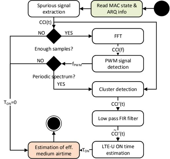
Fig. 6: Flow chart of LTE-U duty cycle detector.
