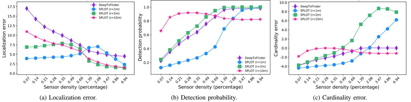
Figure 6. Scenario II: Performance comparison of SPLIT and DeepTxFinder under shadowing and known transmission power.
