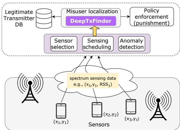
Figure 1. **Spectrum monitoring and misuse detection by crowdsourcing.** DeepTxFinder is part of the solution and its goal is to localize the transmitters according to the sensing data, e.g., received-signal-strength (RSS) measurements, collected from the crowdsensing sensors.
