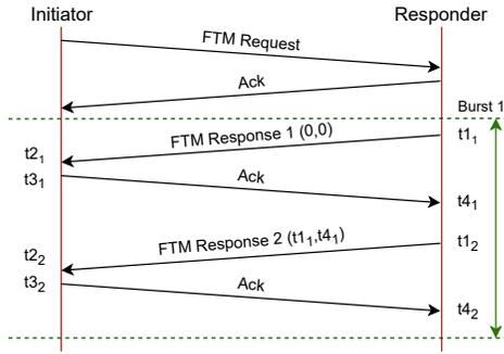
Fig. 1: An FTM exchange with one burst.
