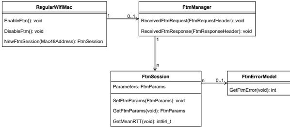
Fig. 4: Class diagram showing the components of FTM-ns3.
