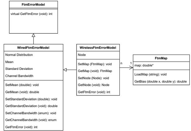
Fig. 5: Class diagram of the ranging error models.
