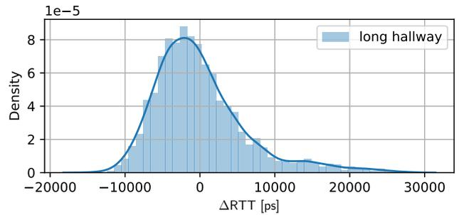
Fig. 3: Ranging error in long hallway (data from [4])
