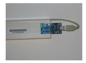
Figure 18: Tmote Sky node connected to a TWIST socket
