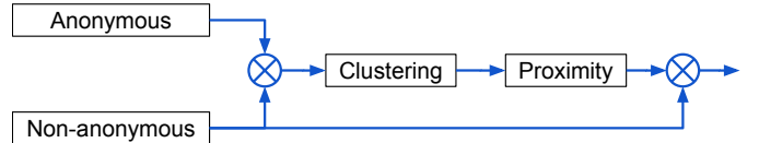
Fig. 6: The localization process. Anonymous and non-anonymous measurements are fused, the heaviest cluster is selected, and finally the non-anonymous measurements are fused and higher weight is given to the particles close to the selected cluster.
